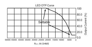
Graphs for reference. The derating limits can be programmed using the Light Touch. In the end application, care must be taken to place the NTC thermistor close to the hottest spot on the LED module.If LED thermal protection is not required the NTC port on the LED power supply connector can be left open.
