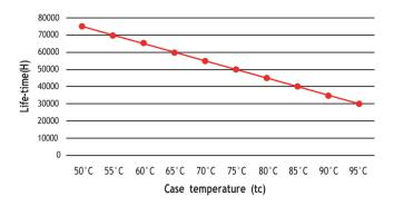
The life-time of the led driver is shown in the figure above (calculated based on the 90% survival rate).
