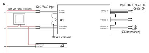
Remark: Only use open push button without indicator light. Maximum cable length between each Unit: 20 meters.
