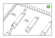
Please do not stack the products. The distance between two products should be>12cm so as not to affect heat dissipation and the lifespan of the products.
