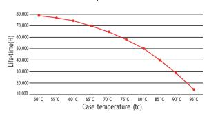
The life-time of the led driver is shown in the figure above (calculated based on the 90% survival rate).
