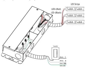
Step 4 UsingTriac ELV wiring diagram
