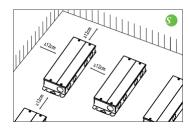
Please do not stack the products. The distance between two products should be>12cm(4.72 in) so as not to affect heat dissipation and the lifespan of the products.
