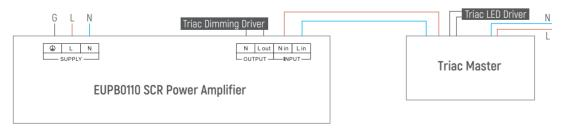
Note: Regardless of the input signal is the leading edge or the trailing edge, EUPB0110 output signal is the leading edge, please note the consistency of the other loop (if any) of the original dimmer.
