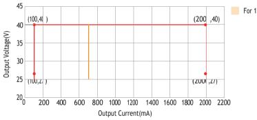
For 100%-1% dimming, set output current ≥ 700mA.
