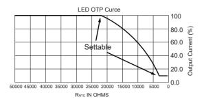
Graphs for reference. The derating limits can be programmed using the Light Touch. In the end application, care must be taken to place the NTC thermistor close to the hottest spot on the LED module.
