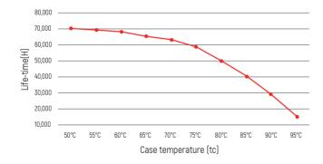
The life-time of the led driver is shown in the figure above (calculated based on the 90% survival rate).
