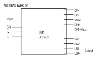
AC input wire (Exposed Wire Length: 300 ±10mm)
